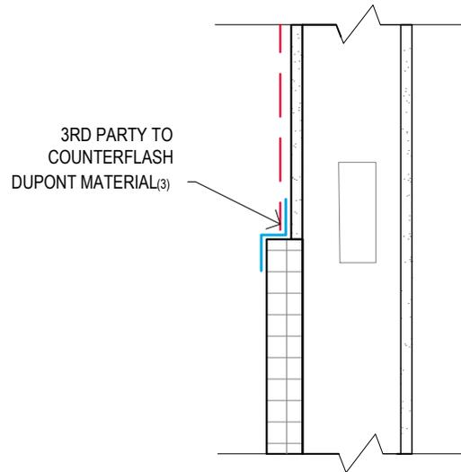
FIG 2: VERTICAL TRANSITION OF OTHER WRB TO THERMAX™ | SECTION
