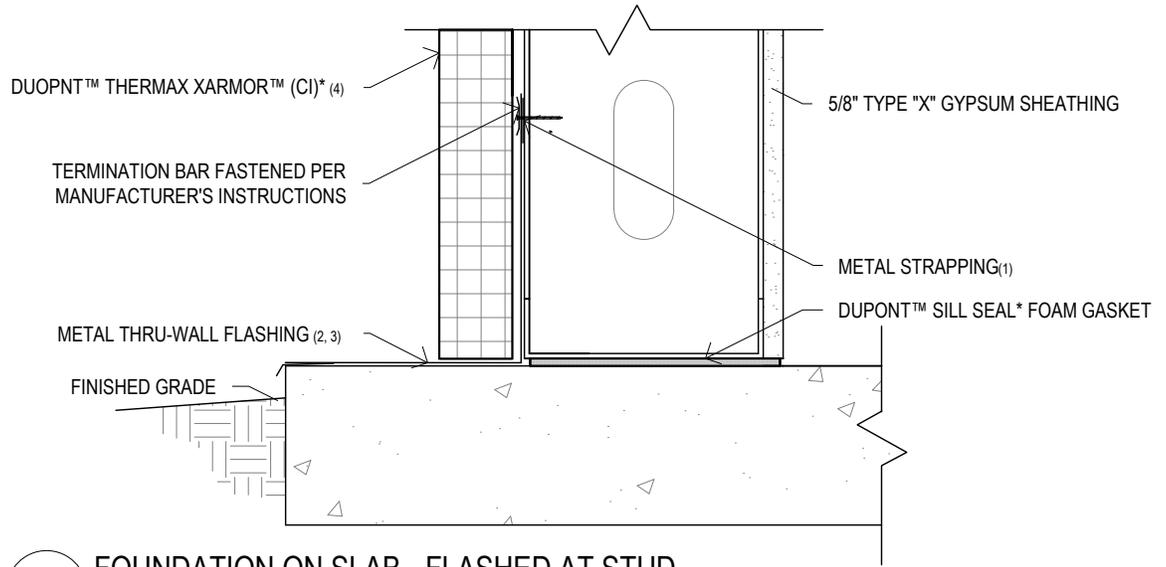
**FOUNDATION ON SLAB - FLASHED AT STUD**
