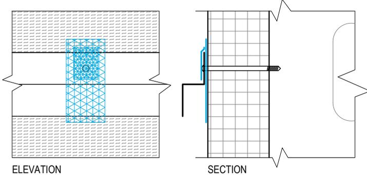
Z-FURRING - VERTICAL USING LIQUIDARMOR™ QS (CURED<sub>3</sub>), CM (CURED<sub>3</sub>), OR LT (WET<sub>4</sub> OR CURED<sub>3</sub>) FLASHING
