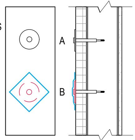
FIG 2: FASTENING FLASHING | ELEV. (L) & SECTION (R)
