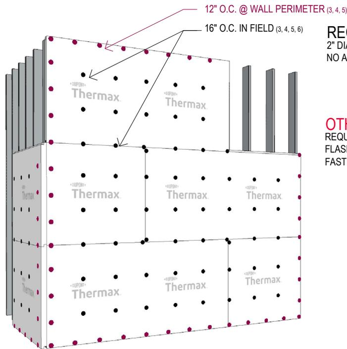
FIG 1: FASTENING PATTERN LAYOUT | ISOMETRIC
