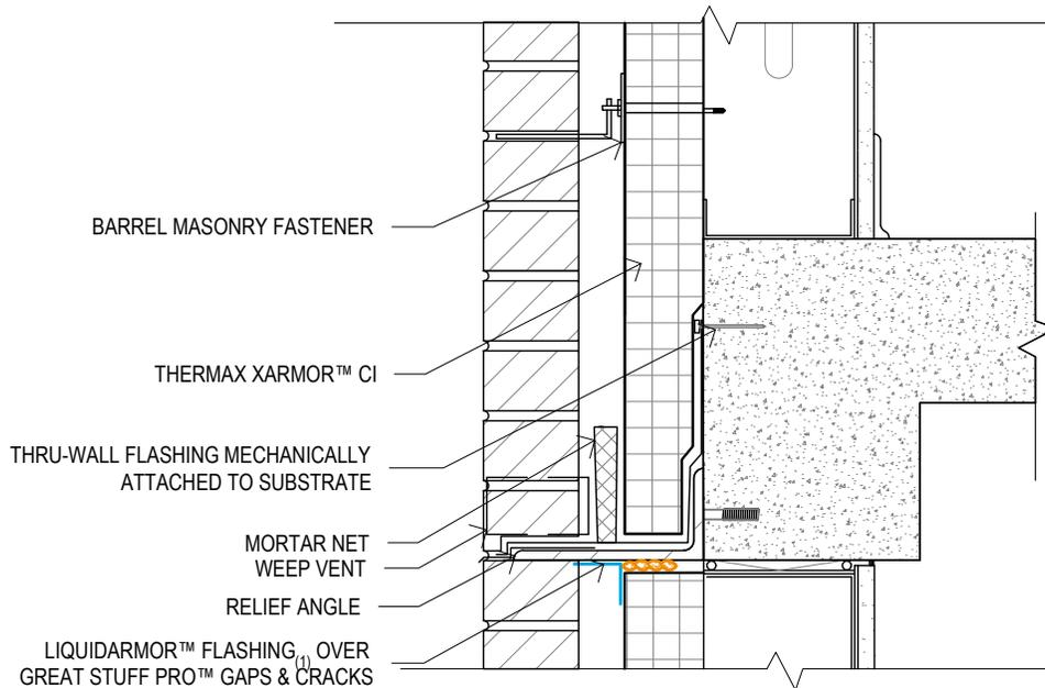
EDGE OF SLAB - FLASHED AT SLAB
