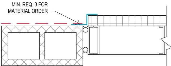
FIG 3: TRANSITION FROM THERMAX™ TO WRB ON CMU | PLAN
