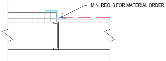
FIG 4: HORIZONTAL TRANSITION OF OTHER WRB TO THERMAX™ | PLAN
