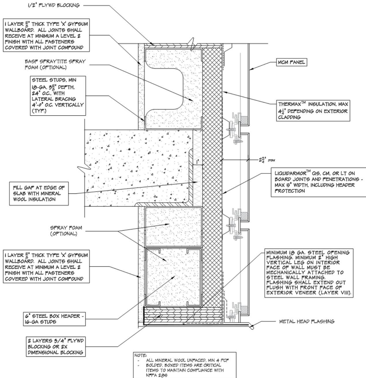
**Figure 6. Required Opening Head Protection When BASF SPRAYTITE® 81206 Spray Foam Is Used in the Cavity (Infill Wall Construction with ACM Façade)**
