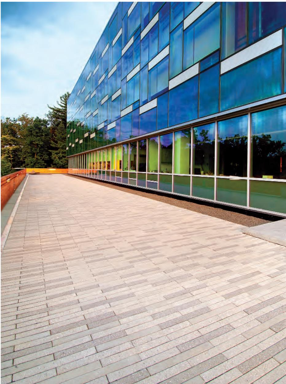
Hidden spacers allow for sand joint interlock. PlankStone® is suggested for pedestrian use only. Hanover® PlankStone® is stocked in Natural/Charcoal, NEW Hickory and NEW Antique Red color blends with a Natural finish. A Tudor® finish, as well as custom aggregates and color blending are available when quantities permit.
