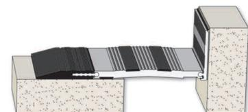
Pedestrian Slab-to-Slab / Movement 0" to 8.5"
