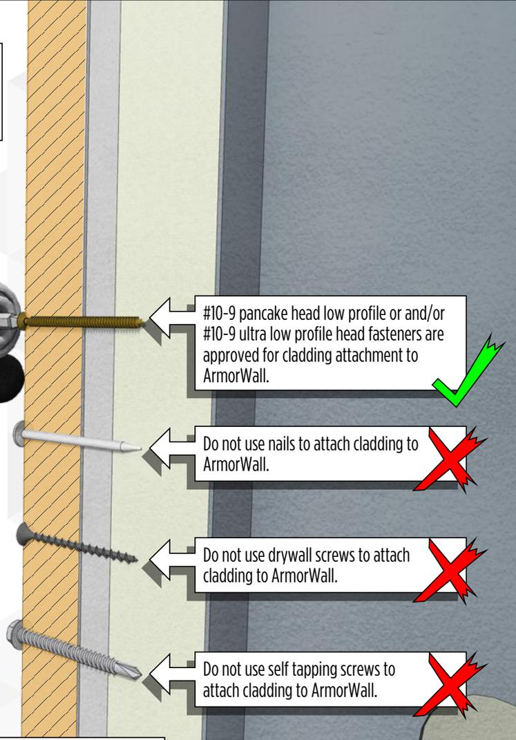
Each attachment screw must penetrate the ArmorWall panel a minimum of 1" after securing claddings, clips, standoffs, and all other attachments. Read the ArmorWall panel data sheets for pullout tolerances.
