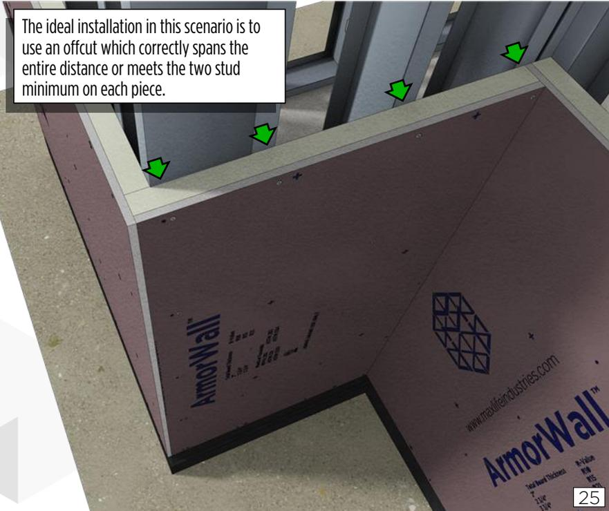
The ideal installation in this scenario is to use an offcut which correctly spans the entire distance or meets the two stud minimum on each piece.
