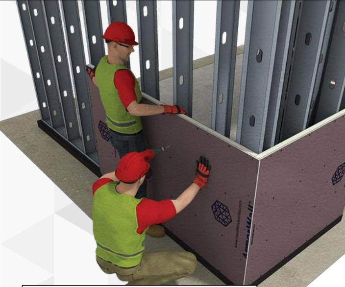
Continue rounding the next corner using the same outside corner steps having prepared the panel for the weave joint.
