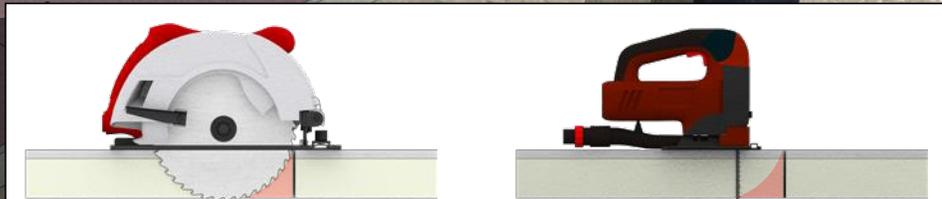
It is recommend to finish the inside corners after the circular saw using a jig saw tool.
