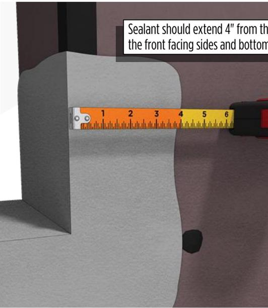
Sealant should extend 4" from the interior on to the front facing sides and bottom of the panel.
