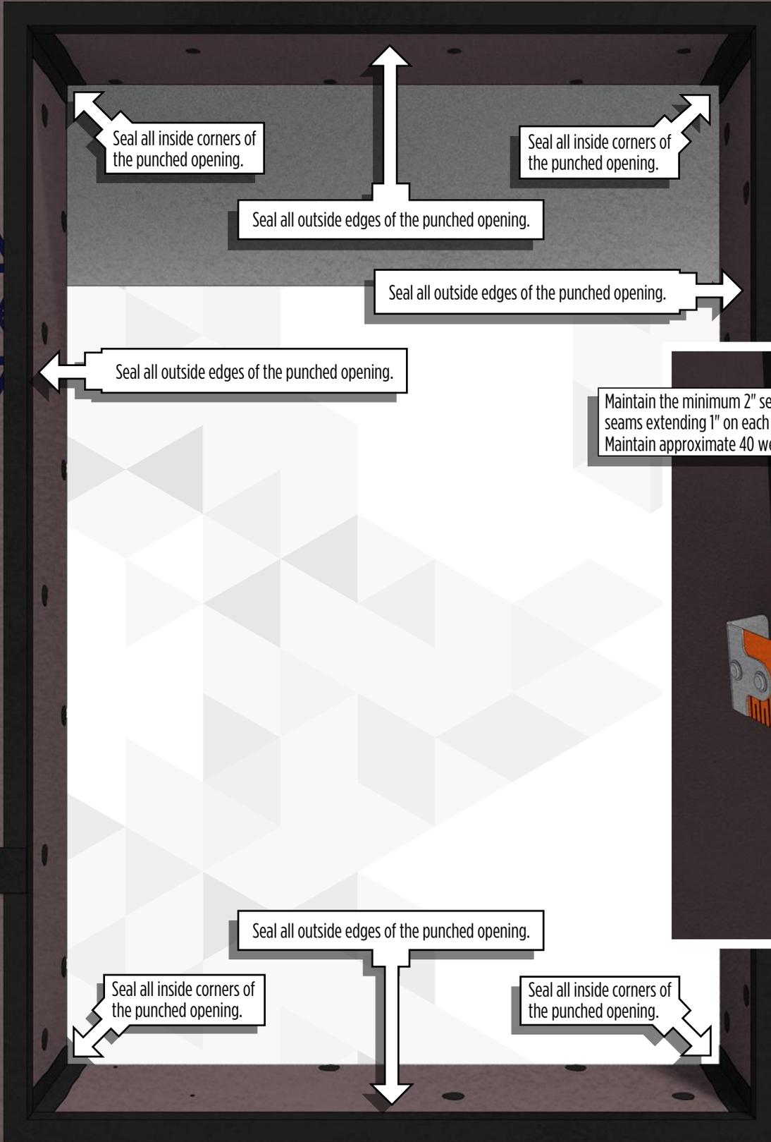
Maintain the minimum 2" sealant coverage at seams extending 1" on each face after striking. Maintain approximate 40 wet mil thickness.
