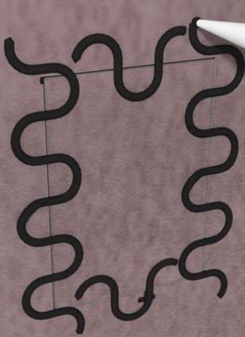
Seal the measured and cut panel piece in place using ArmorSeal Sealant (Gunnable Grade). Take care to insure sealant spans a minimum 1" on each face of the seam when struck, 2" total width, and to achieve approximately a 40 wet mil thickness free of voids and holidays.
