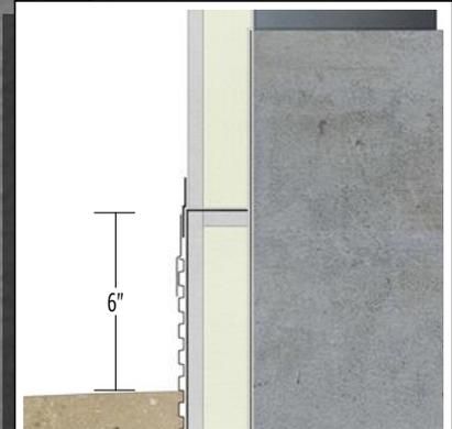
ArmorWall Below Grade (BG) is manufactured to make the transition to the above grade panels effortless as it already has built-in returns. When transitioning, you only require the typical 2" lap sealant between the panels. When installing above grade always follow exterior finish clearance guidelines and installation procedures.
