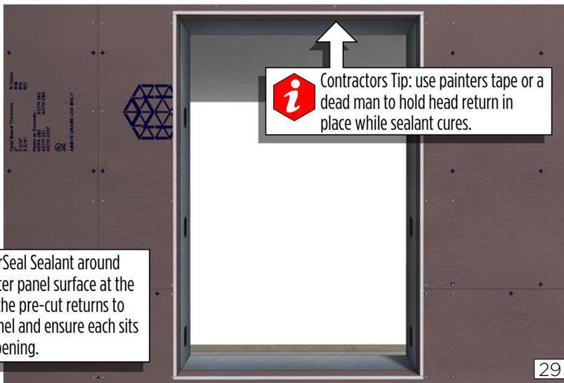
**i** Contractors Tip: use painters tape or a dead man to hold head return in place while sealant cures.
