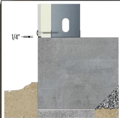
ArmorWall can be installed flush with the foundation. In this case, offset the base of the panel 1/4" from the foundation and install a backer rod and sealant around the entire perimeter as necessary.
