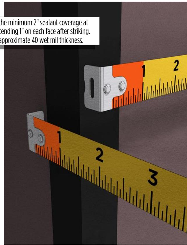
Gaps up to 1/8" in width receive the standard 2" wide joint seam spanning 1" on each surface face.
