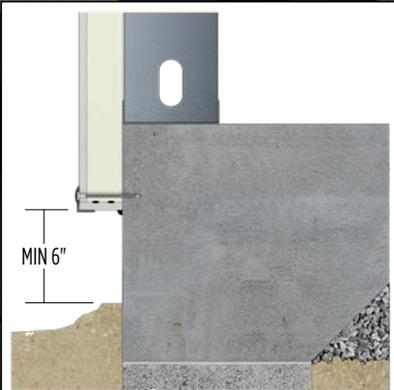
ArmorWall can be installed to be in front of the foundation slab. There is an additional step of adding a Plus return cap measured the thickness of the panel as well as a bead of ArmorSeal Sealant at the base of the panel where it meets the concrete. When installing above grade always follow exterior finish clearance guidelines and installation procedures.
