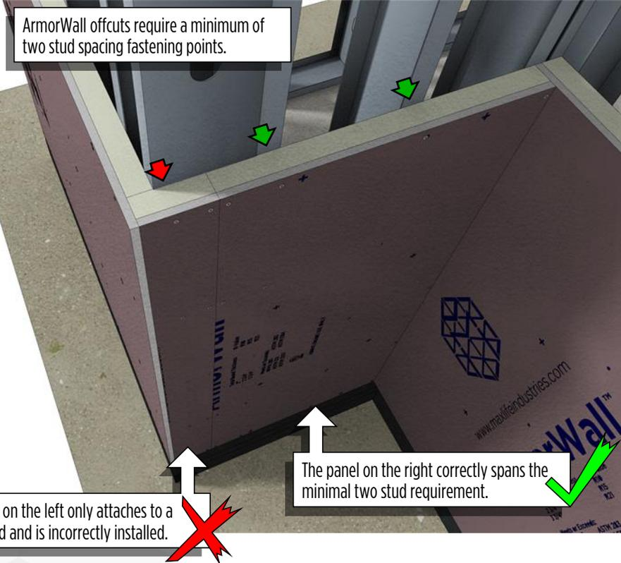
ArmorWall offcuts require a minimum of two stud spacing fastening points.
