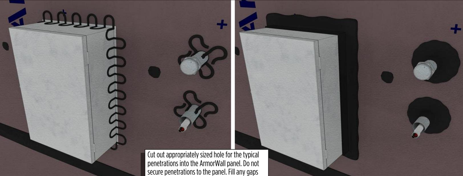
Cut out appropriately sized hole for the typical penetrations into the ArmorWall panel. Do not secure penetrations to the panel. Fill any gaps 1/8" or greater resulting from oversized holes with appropriately sized compressible backer rod. Apply ArmorSeal Sealant to the penetration at the hole and strike to achieve approximately a 40 wet mil thickness and to ensure free from voids or holidays.
