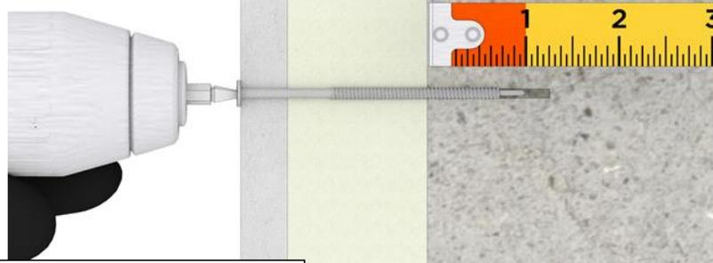
Fasten #14-13 self-tapping screws to be proud of the ArmorWall surface. Where countersinking the screws is preferred, always use a countersink bit. Do not countersink screws in high wind zones.
