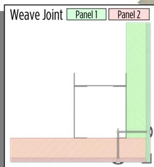
Fasten next panel around the outside corner in to the pocketed extension to complete the weave joint.
