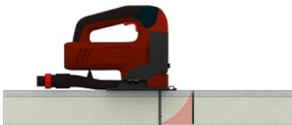
It is recommend to finish the inside corners after the circular saw using a jig saw tool.
