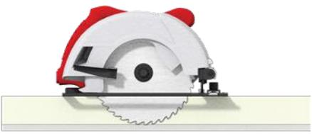
Set the depth of your saw to only cut the foam insulation.
