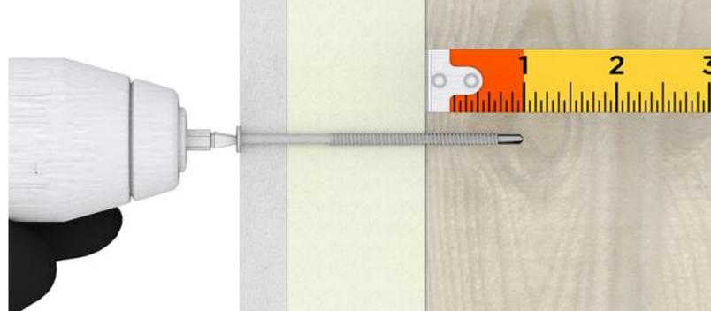
Fasten #14-13 self-tapping screws to be proud of the ArmorWall surface. Where countersinking the screws is preferred, always use a countersink bit. Do not countersink screws in high wind zones.
