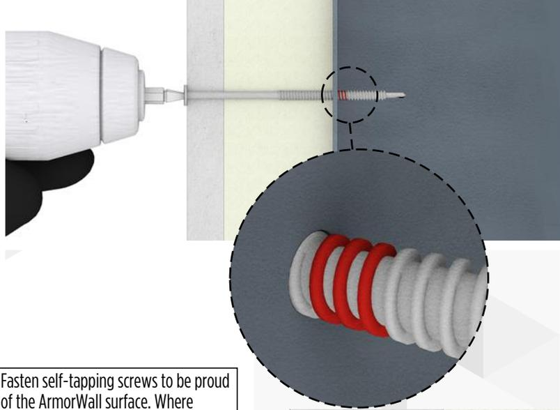
Fasten self-tapping screws to be proud of the ArmorWall surface. Where countersinking the screws is preferred, always use a countersink bit. Do not countersink screws in high wind zones.
