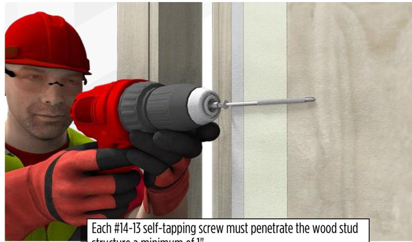
Each #14-13 self-tapping screw must penetrate the wood stud structure a minimum of 1".
