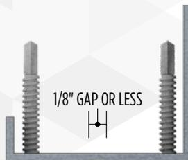
Fill gaps greater than 1/8" to 3/4" with low rise foam (illustrated) or compressible insulation filler followed by a compressed backer rod and ArmorSeal Sealant. Seams and gaps receive the standard 2" wide joint seam spanning 1" on each surface face.
