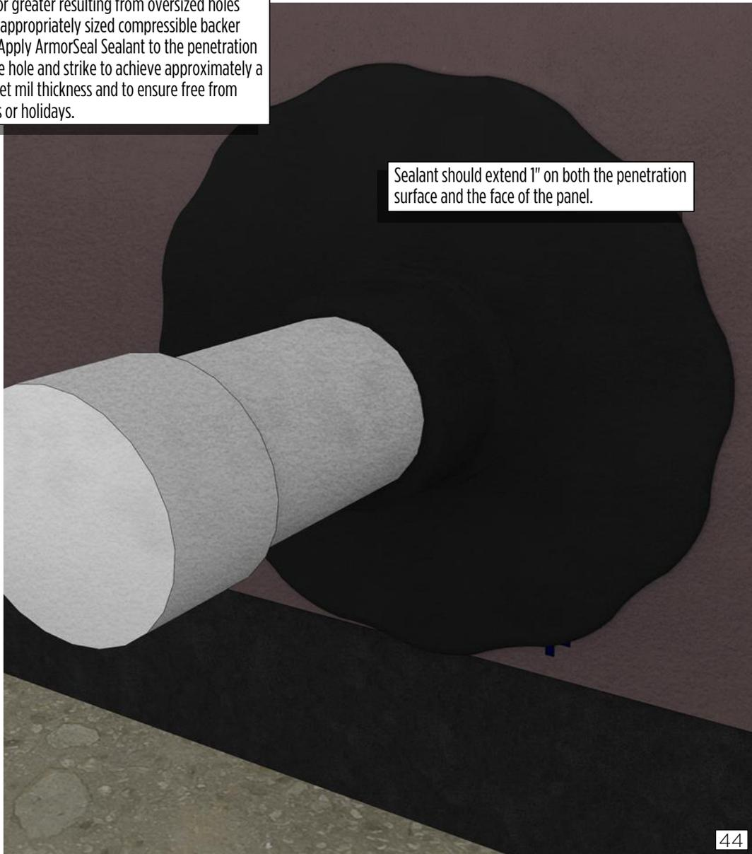
Sealant should extend 1" on both the penetration surface and the face of the panel.
