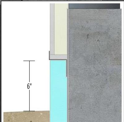
When transitioning from ArmorWall Plus to a traditional below grade insulation you must cap off the edge of the panel with a return. The corner lap sealant then must transition back to the foundation waterproofing. When installing above grade always follow exterior finish clearance guidelines and installation procedures.
